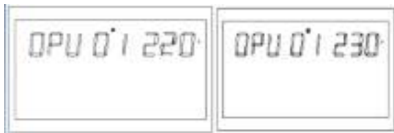
Figure 1-18 Output Voltage Setting
