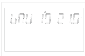
Figure 1-36 Battery Low Voltage cut off Point Setting Page
